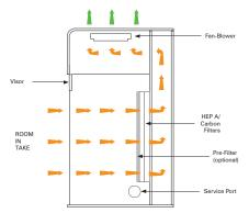
Room air enters the cabinet passing the operator and horizontally through the rear mesh back panel, up the back of the cabinet and through the filtration system returning clean air back into the laboratory.
