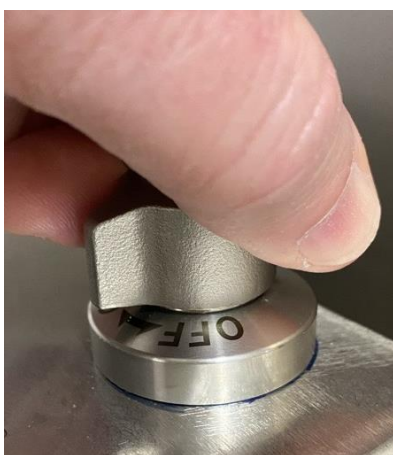
Shaker platform fastener locked position
