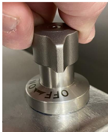
Shaker platform fastener unlocked position
